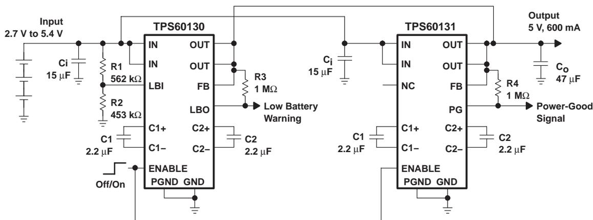
Figure 25. Paralleling of Two TPS6013x Charge Pumps
